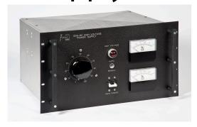
The GDS100 output is variac controlled with remote On/Off capability. There are two (2) safety interlocks available (door and vacuum) to protect both the operators and the hardware.
